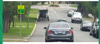
The Shire recently installed solar powered LED speed signs in View and Leake Streets. These devices measure, then clearly display each vehicle's speed as it approaches the unit.
