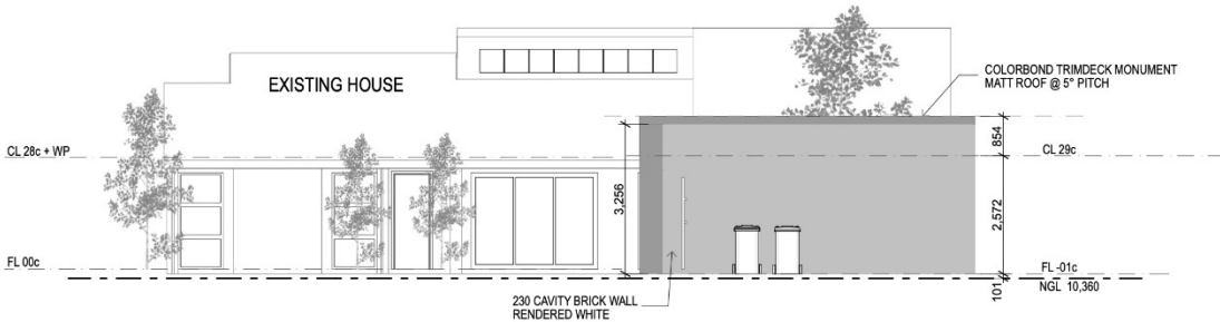
NORTH ELEVATION SCALE 1:100
