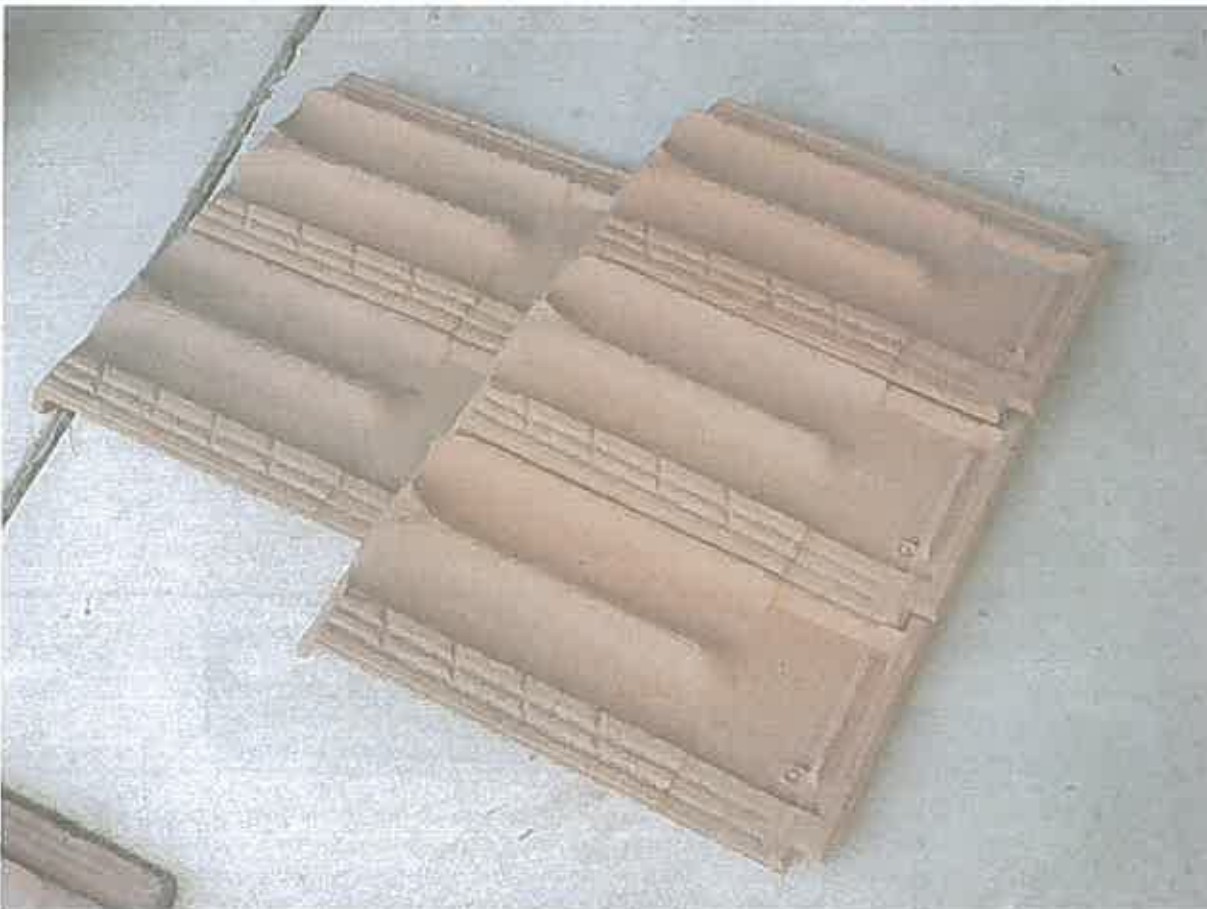
Figure 4: Sample of contemporary unglazed terracotta Marseille tiles from a reputable supplier in France. Colours, which are readily available in their product range, are mixed in the attempt to match the gradation and colour range of the existing roof.
